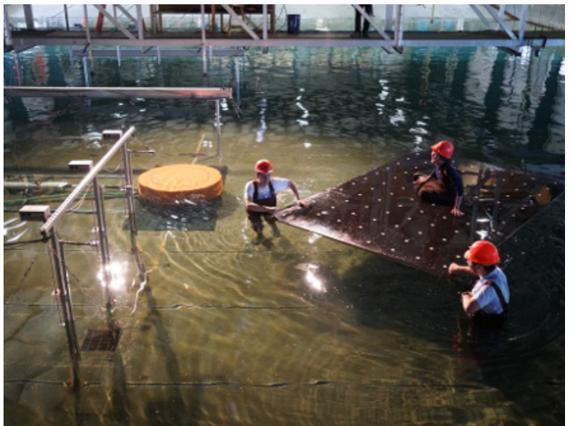
NSF REU students have fun rafting/floating the dotted calibration board on top of the submerged orange volcanic tsunami generator. The calibration board is used for the stereo, video-based, 3D surface reconstruction. (Photo: Hermann Fritz, Georgia Tech)
