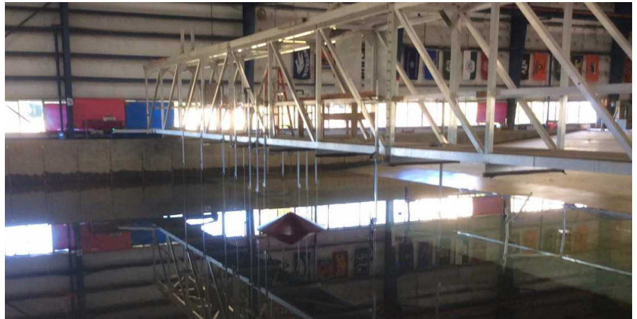
Experimental setup for water depth of 0.5m. Full conical island installed in basin. Vertical structures are wave gauges mounted to the aluminum bridge spanning the basin.
