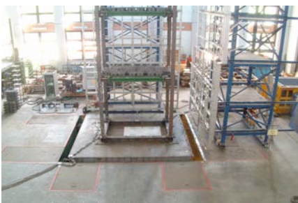
3D earthquake simulator (5m x 5m)
