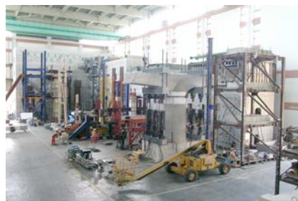
L-shape reaction wall and strong floor
